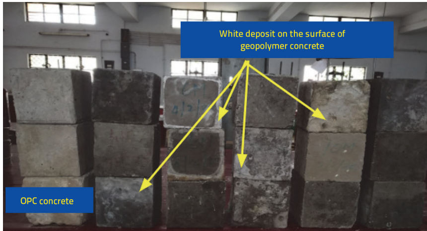
Figure 9. Specimen after sodium sulphate immersion
