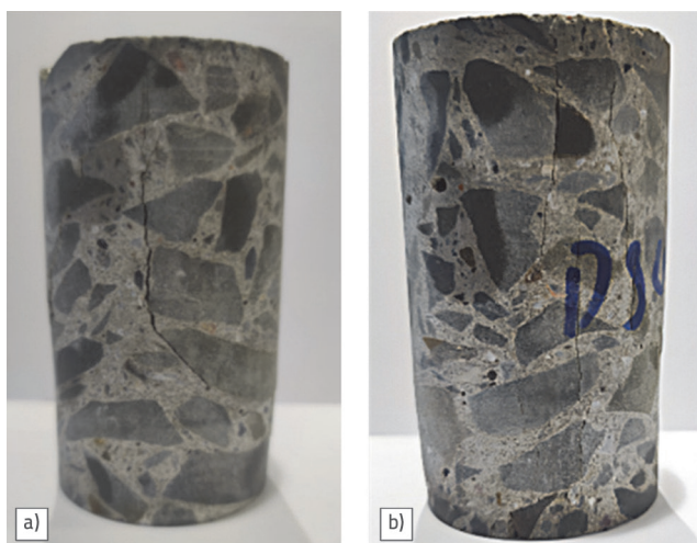
Figure 11. Failure mode of rock-like materials under different freeze-thaw cycles: a) 0 freeze-thaw cycles; b) 30 freeze-thaw cycles
