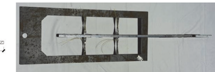
Figure 9. Two-stage damper (D-2) size and physical diagram
