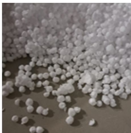
Figure 2. Cracked beads of mechanically recycled EPS
