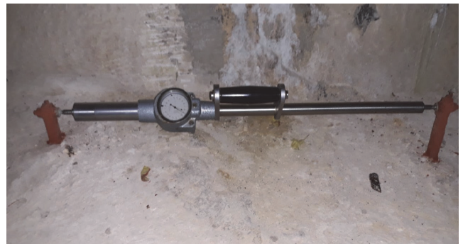
Figure 3. Joint meter located at the dam crest (cantilever 9) where the measurements used for the neural network were obtained
