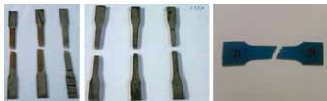
Figure 6. Specimens with sheet thicknesses of 2 mm (T2-L), 4 mm (T4-L) and 0.85 mm (T1)
