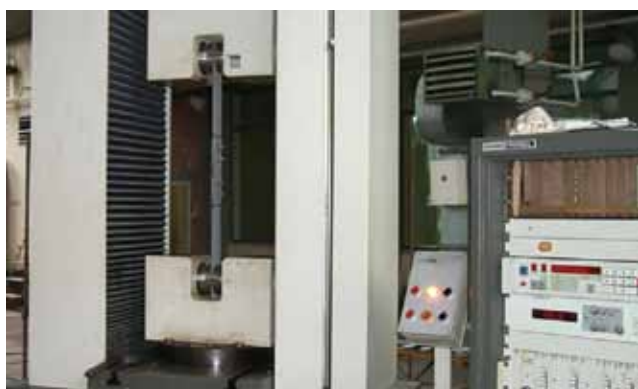
Figure 5. Electronic cutting machine RM400, 400 kN in capacity
