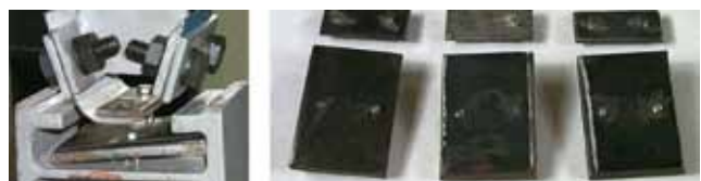
Figure 19. Failure of self-tapping screws loaded in tension
