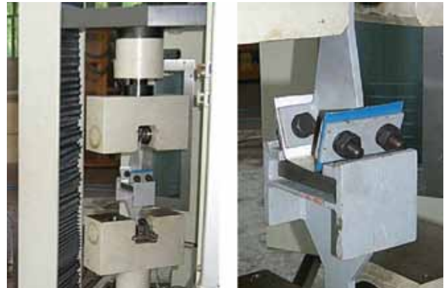
Figure 16. Testing specimens in connections loaded in tension
