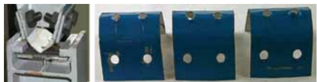
Figure 18. Failure of the self-tapping screw head by pull through the profiled sheet
