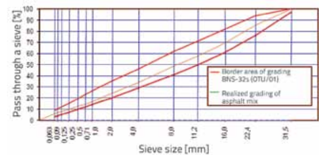
Figure 4. Grading of asphalt mix with 20 % of recycled asphalt
